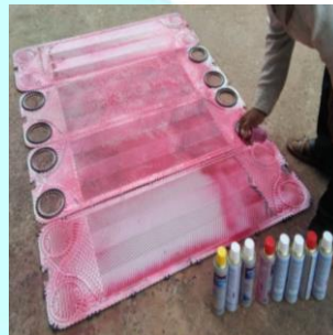
DP Testing of Heat Transfer Plate
