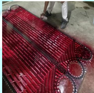
DP Testing of Heat Transfer Plate
